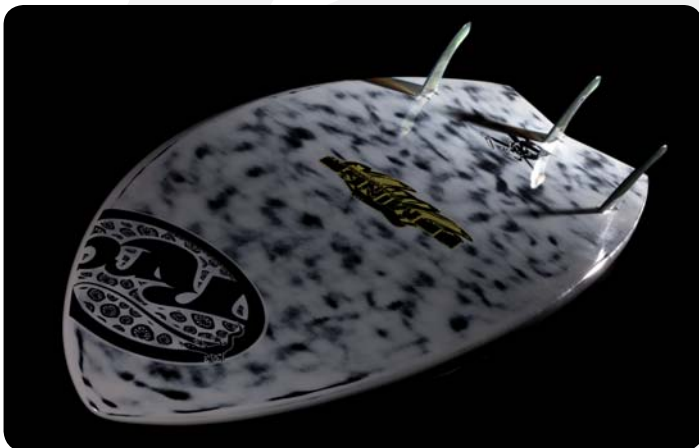
Plain flat hull with slight V rail to rail configuration and very low entry on the nose.
